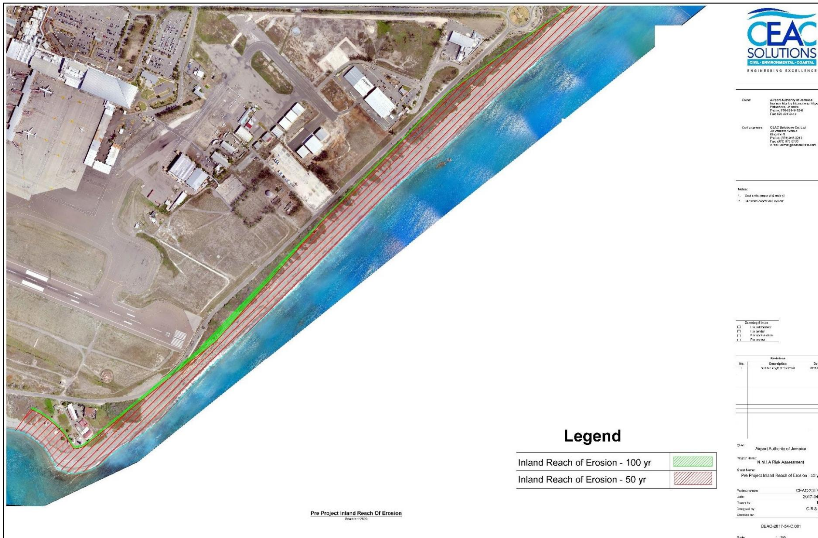
Figure 3-4: Erosion for the 50 and 100 year storm event
