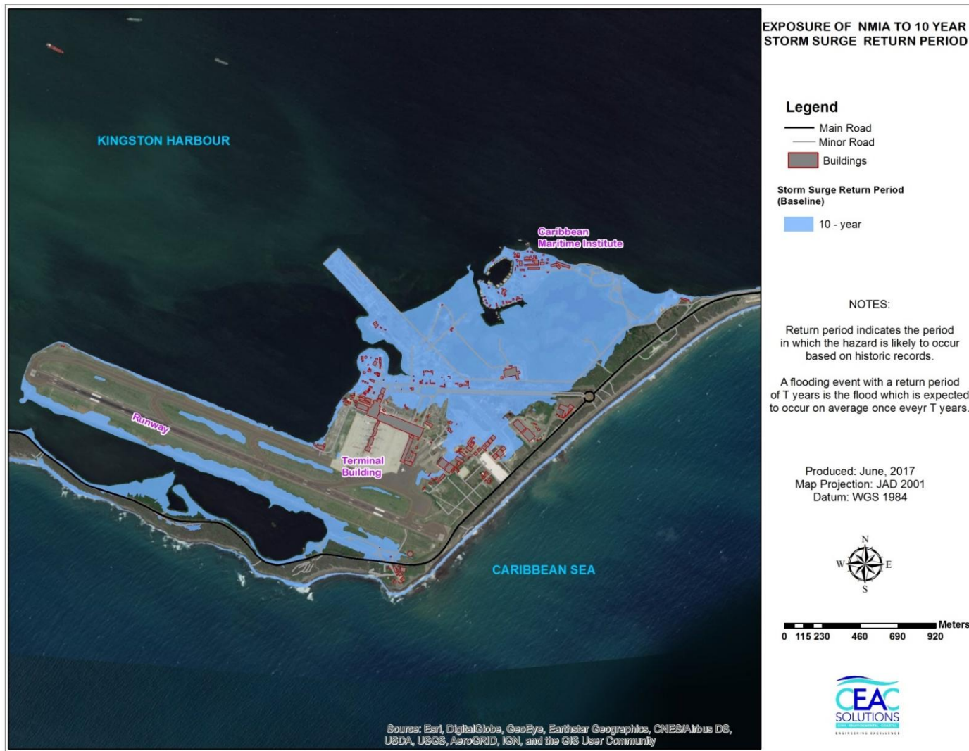
Figure 3-1: Exposure of Airport Assets to 10 Year Storm Surge Return Period
