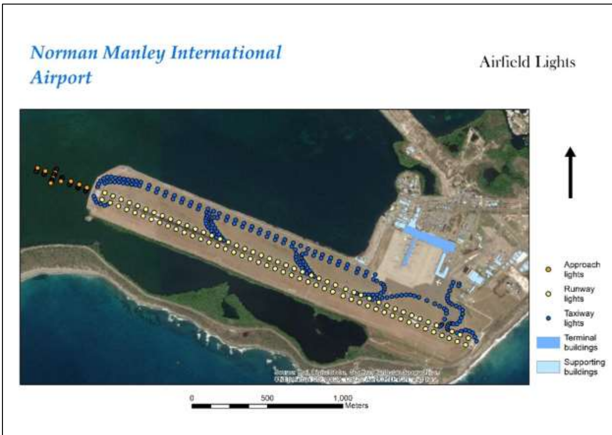
Figure 2.19 The Distribution of Airfield Lights Airside
