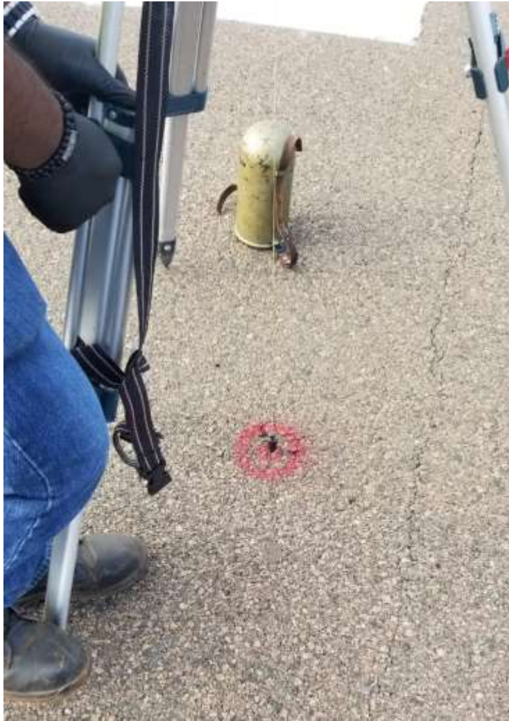
Figure 5.22: Typical survey mark at ends of runway alignment
