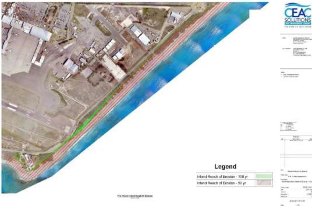
Figure 6.6 Erosion for the 50- and 100-year storm event
