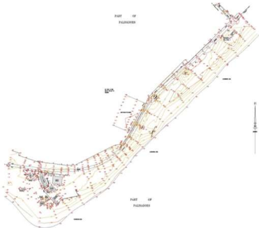
Figure 6.11 Topographic survey points along the 1km project area
