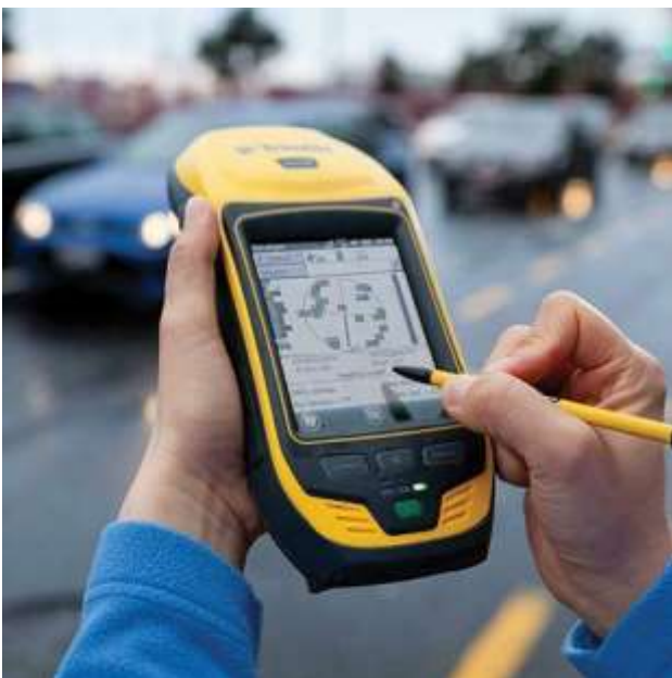
Figure 2.30 Trimble Geo7x handheld GPS device
