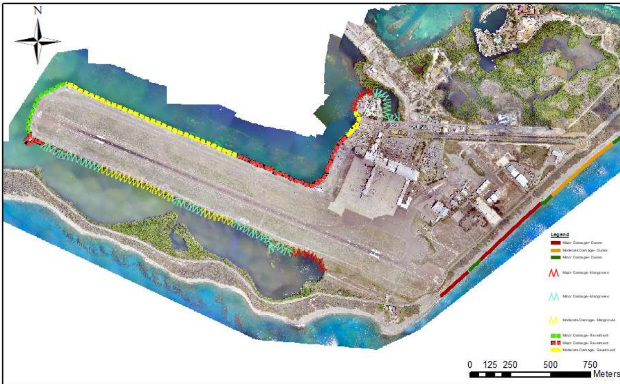
Figure 6.60 Aerial imagery of the section of the NMIA Airport facility showing the shoreline. The sections with the dashed symbology represent the revetment, the zig zag pattern section represents mangroves and the solid lines are the dunes. The red represents portions of the shoreline that needs rehabilitation. The yellow sections represent needs repairs to the shoreline and the green sections shows minor damages.
