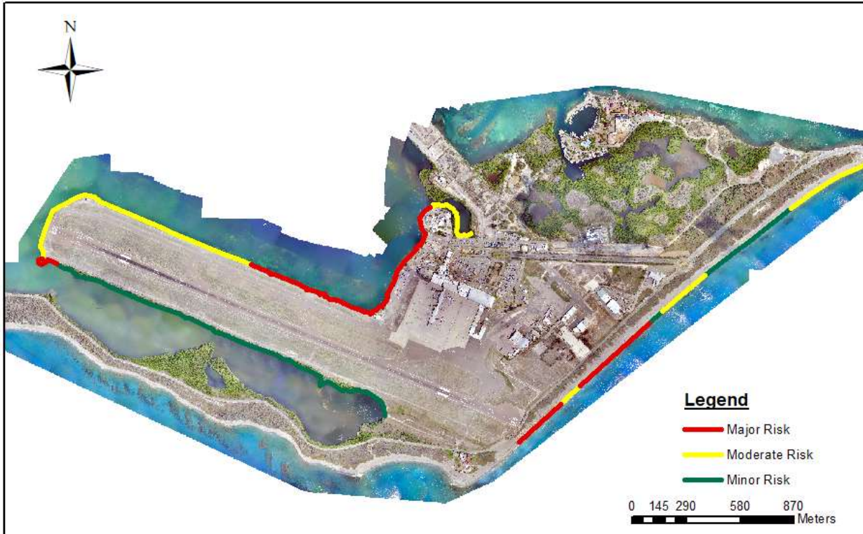
Figure 6.61 Aerial imagery of the section of the NMIA Airport facility showing the shoreline. The sections highlighted in red represents portions of the shoreline that have major damages. The yellow sections represents moderate damage to the shoreline and the green sections shows minor damages.
