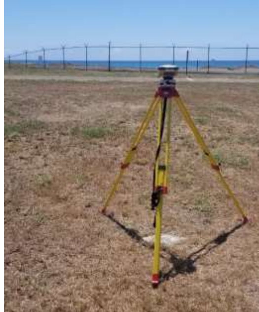
Figure 5.25 Image of Base Station Receiver Setup
