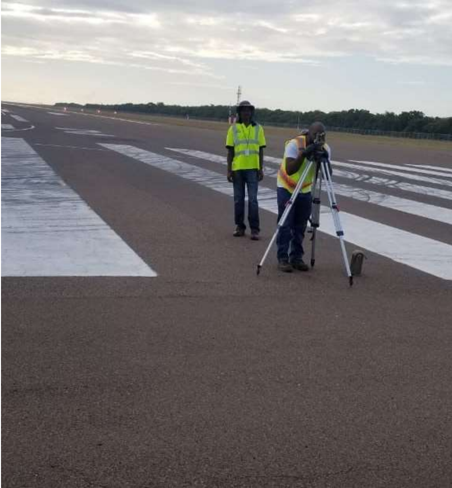
Figure 5.23: Wild T0 Instrument Setup at runway 12
