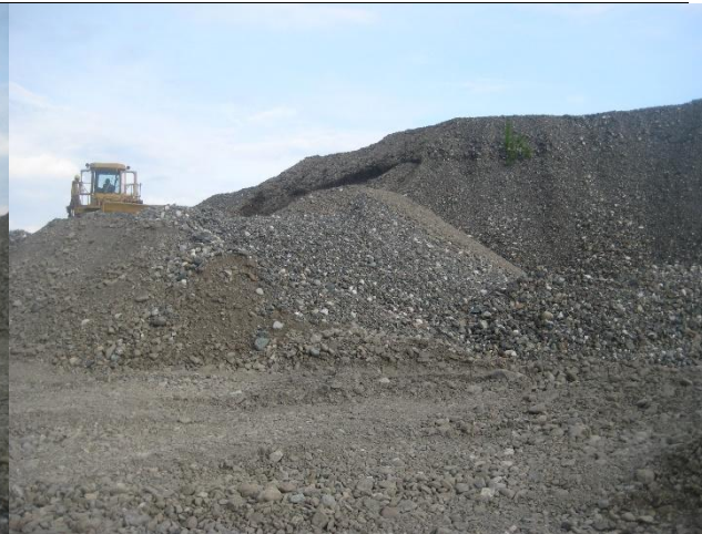
Plate 2.8. Stockpile of material at quarry previously removed from river bed.
