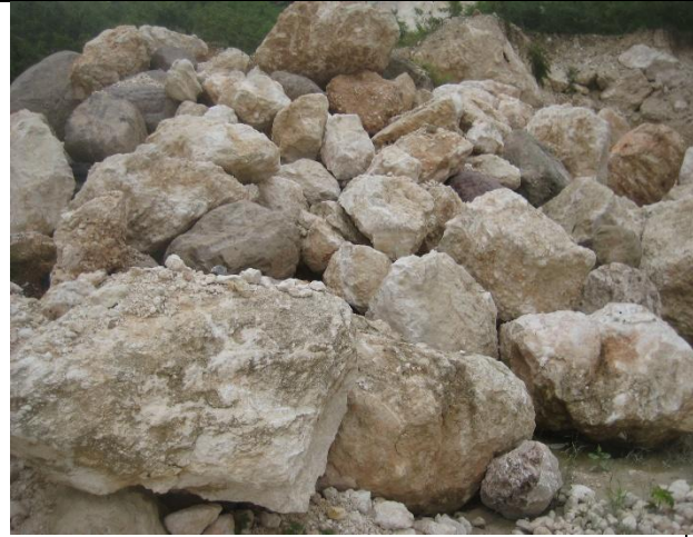
Plate 2.5. Picture shows stones stockpiled at Black's Quarry. The picture shows the soft brittle material which makes up some of these stones.
