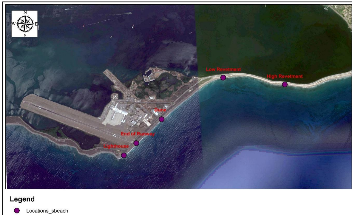
Figure 5.1 Location of the profile lines used in the storm surge model to determine the shoreline response to a 50 and 100 year storm event.
