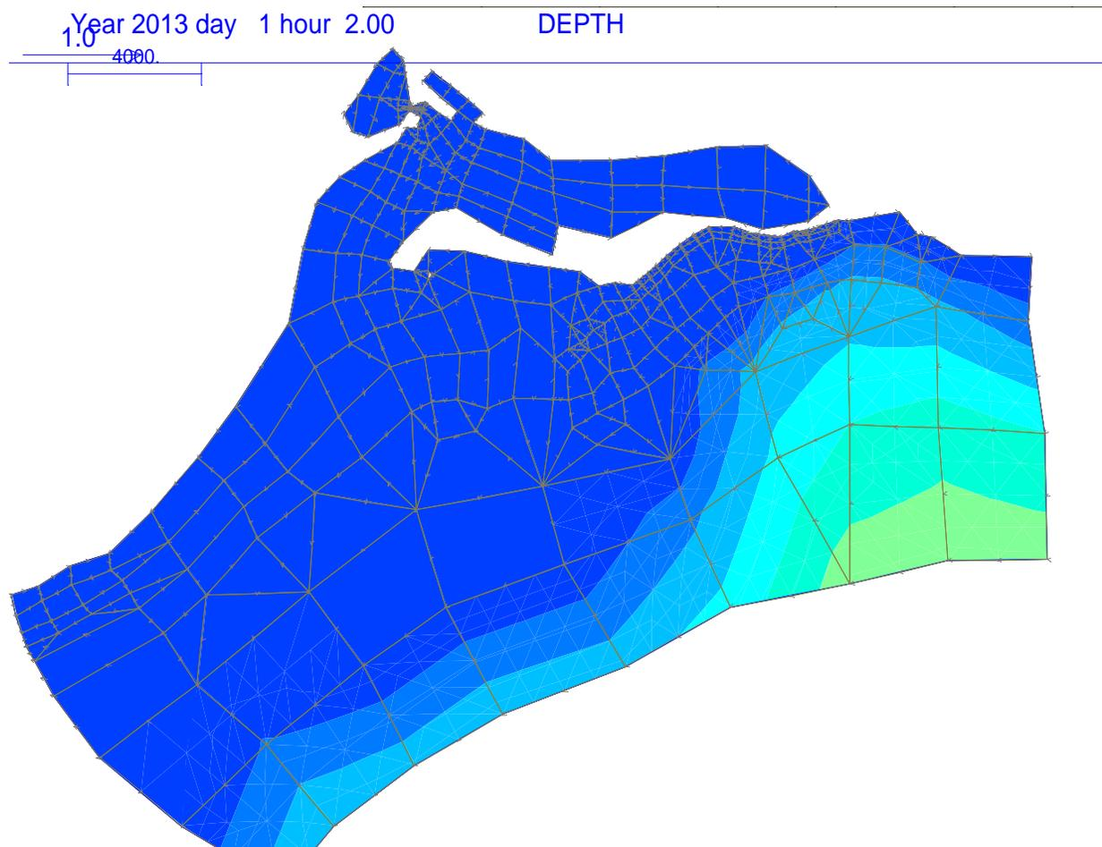
**Figure 5.1 Overview of entire Finite Element Mesh used for this project showing depth in meters**
