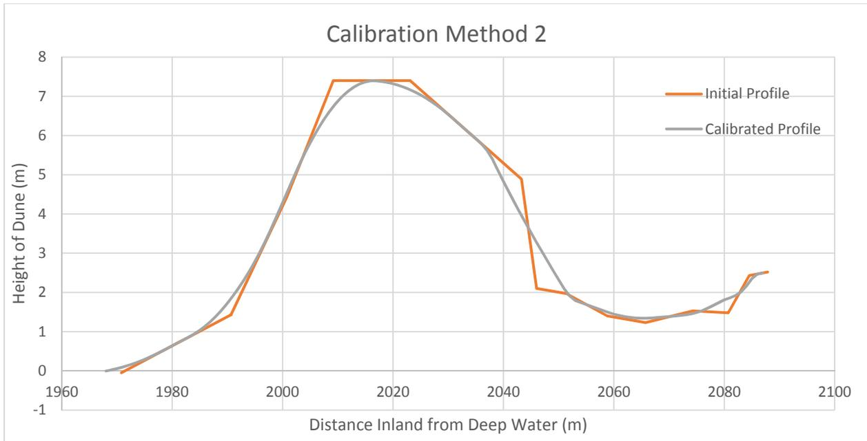
**Figure 4.6 Calibration results comparing observed sand dune movement versus model predictions**
