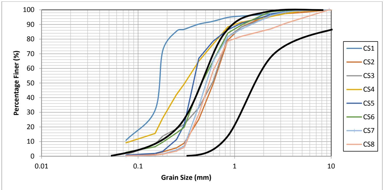
**Figure 2.30 Graph showing the grain size for the sand reserve samples with the upper and lower bounds for the shoreline samples (in black) indicating where suitable sand is located**
