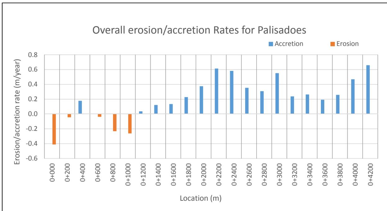
Figure 4.4 Graph showing the overall displacements of the shoreline about the 1968 shoreline for Palisadoes between 1991 and 2013. This graph indicates that the Palisadoes is in accretion mode.
