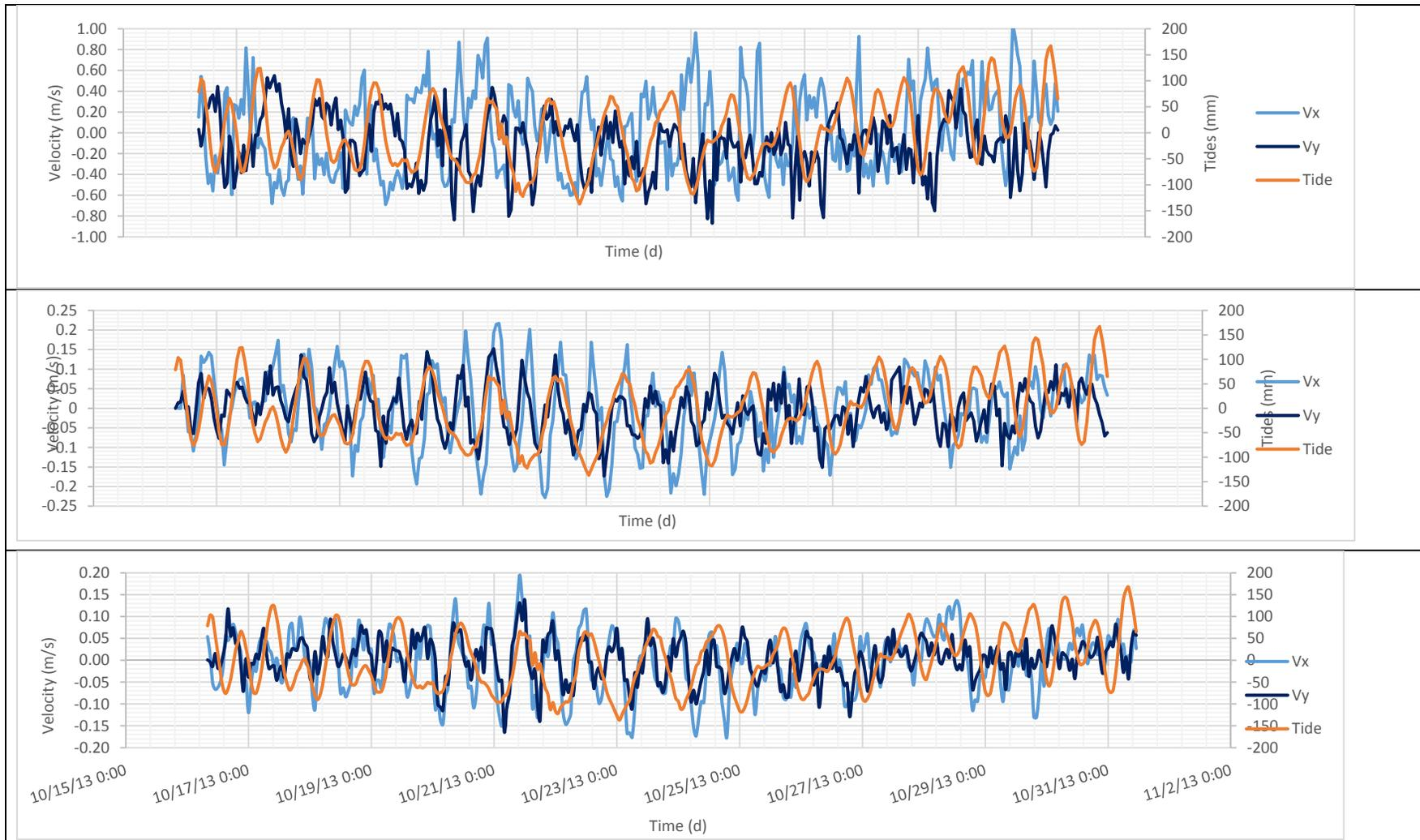
**Table 2-1 Current velocities and tide recordings during the first ADCP deployment of the centre of Palisadoes inline with the burrow area for the surface (top panel), mid depth and sea floor (bottom panel) respectively**
