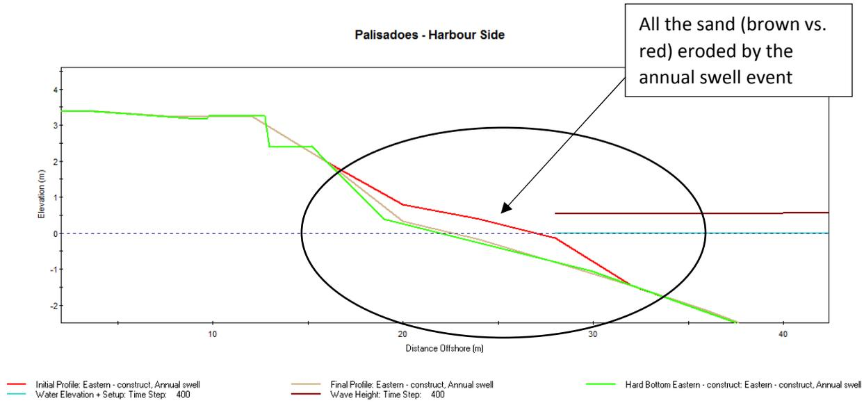
**Figure 4.14 SBEACH results showing the sand placement for mangrove nourishment at the eastern section of the harbour. The sand is placed at a 1: 10 slope and it is almost completely eroded after the passing of the annual swell event**
