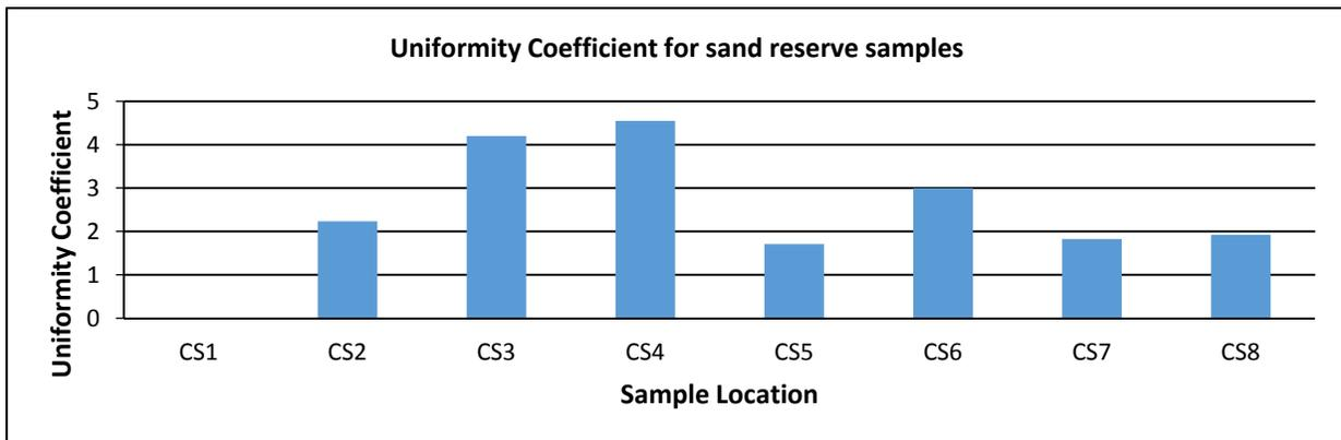
Figure 2.23 Uniformity coefficient for the samples from the sand reserve
