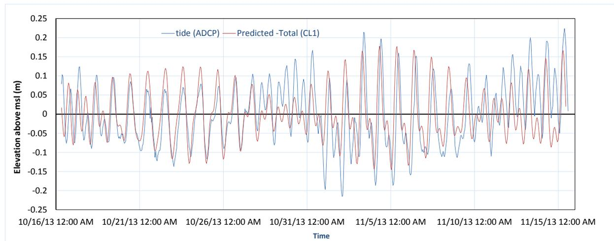
**Figure 2.5 Measured and predicted tidal signature for the Palisadoes for the period October 16, 2013 to November 15, 2013**
