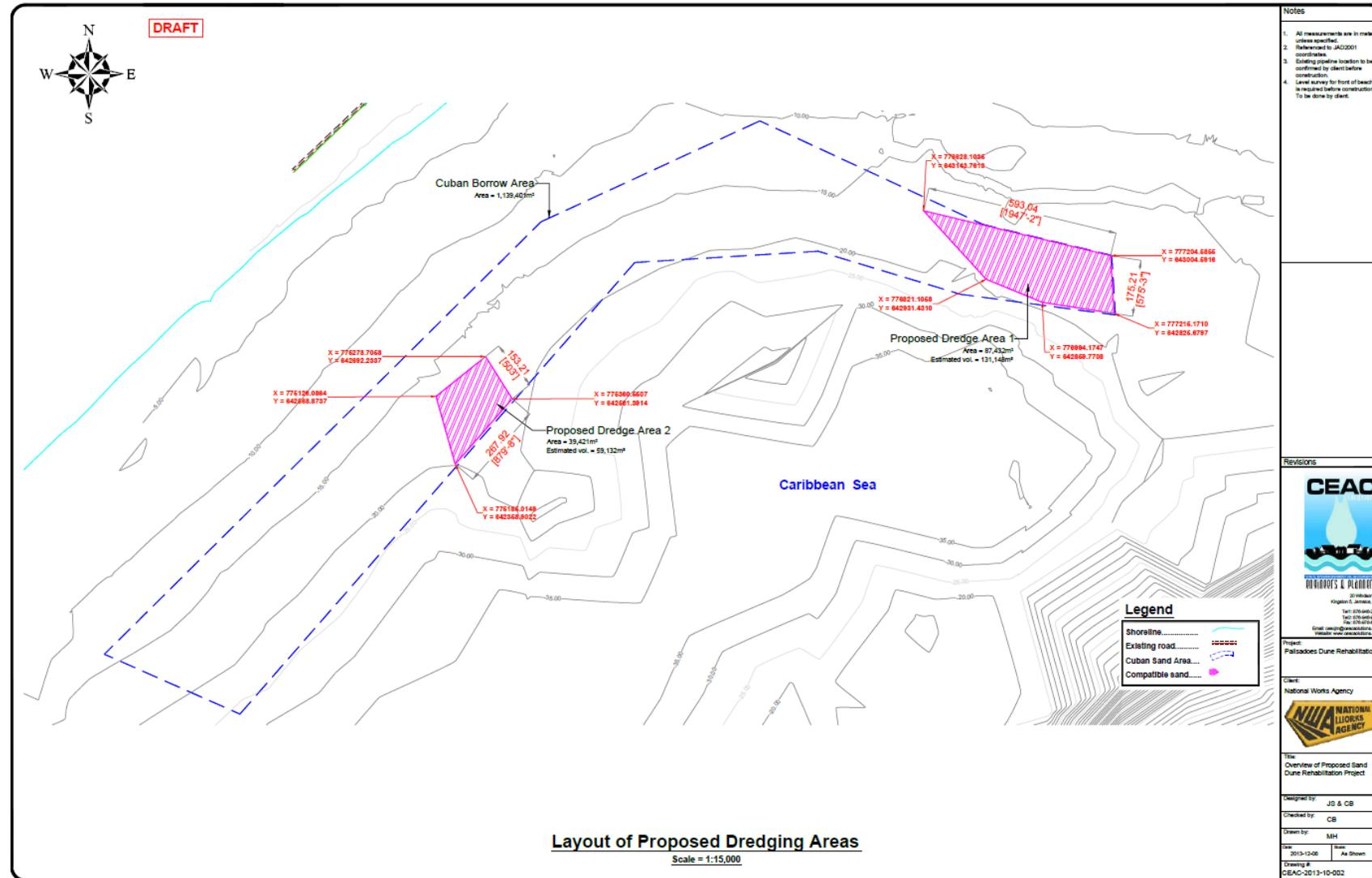
Figure 2.31 Location of sand with a mean grain size of between 0.5 – 0.7 mm within the borrow area. This area should be dredged to a depth of 1.5 m to obtain the required volume
