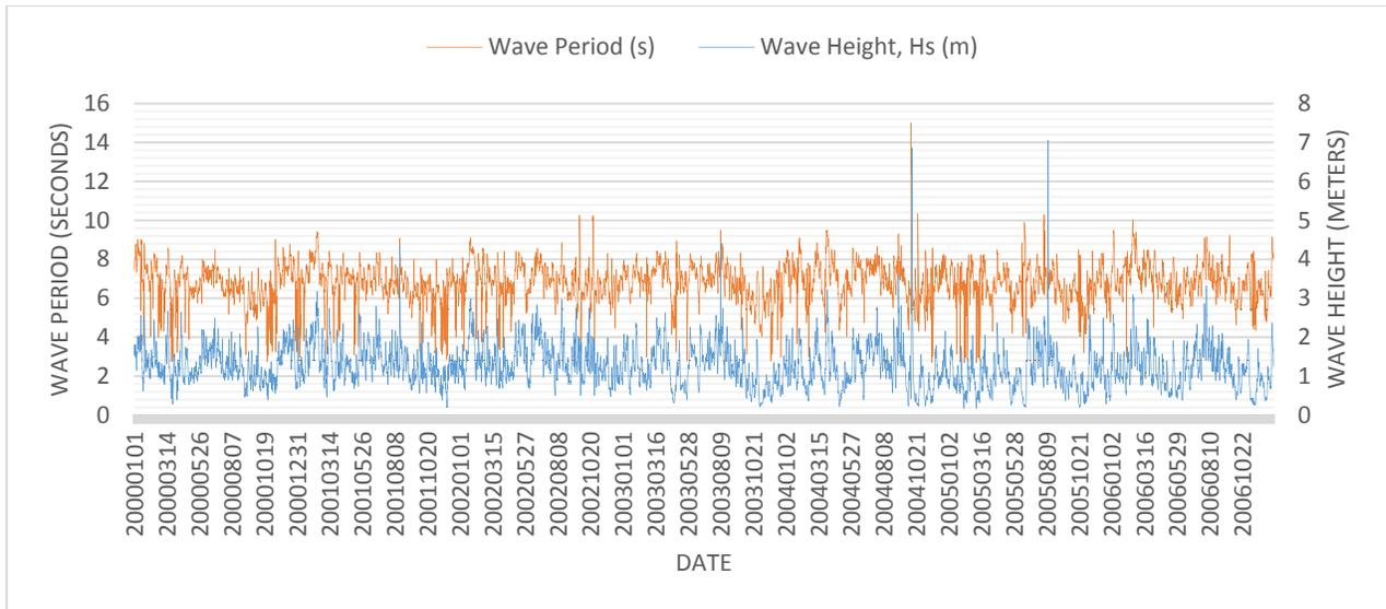
**Figure 4.17 NOAA grib wave data for 2000 - 2006 that was used in sediment transport modeling for the Caribbean Sea side**
