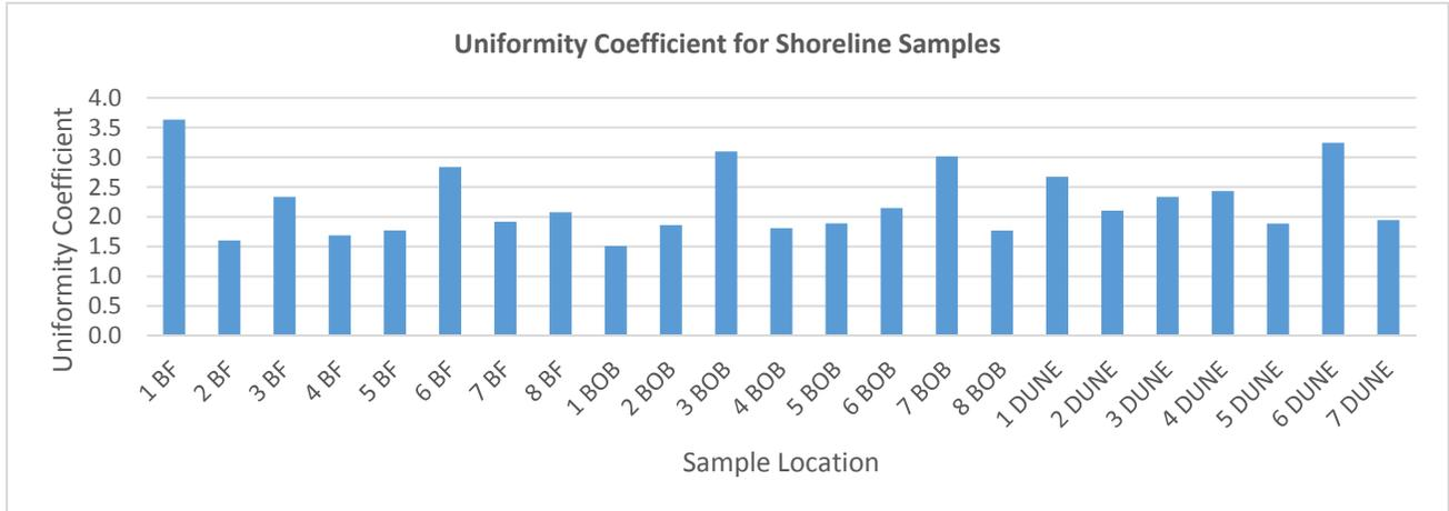
Figure 2.22 Uniformity coefficient for the sand samples taken from the shoreline
