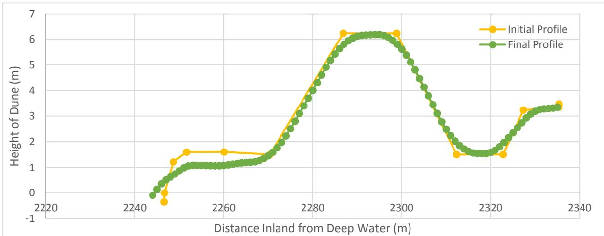
**Figure 4.8 Simulation results comparing pre and post sand dune erosion predictions during 50 year event**
