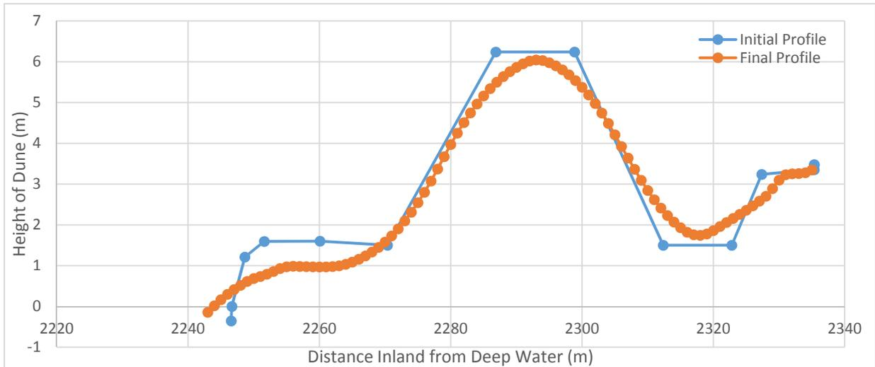
**Figure 4.9 Simulation results comparing pre and post sand dune erosion predictions during 100 year event**
