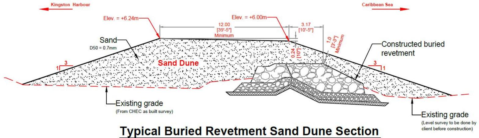
Figure 4.10 Typical section of the sand dune to be placed over the buried revetment along the Caribbean Sea side of the Palisadoes
