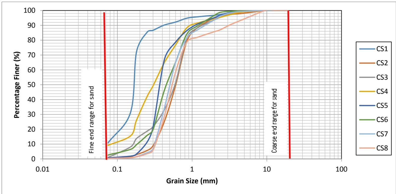
Figure 2.21 Graph showing the grain size plots for the sand samples from the sand reserve (borrow area)
