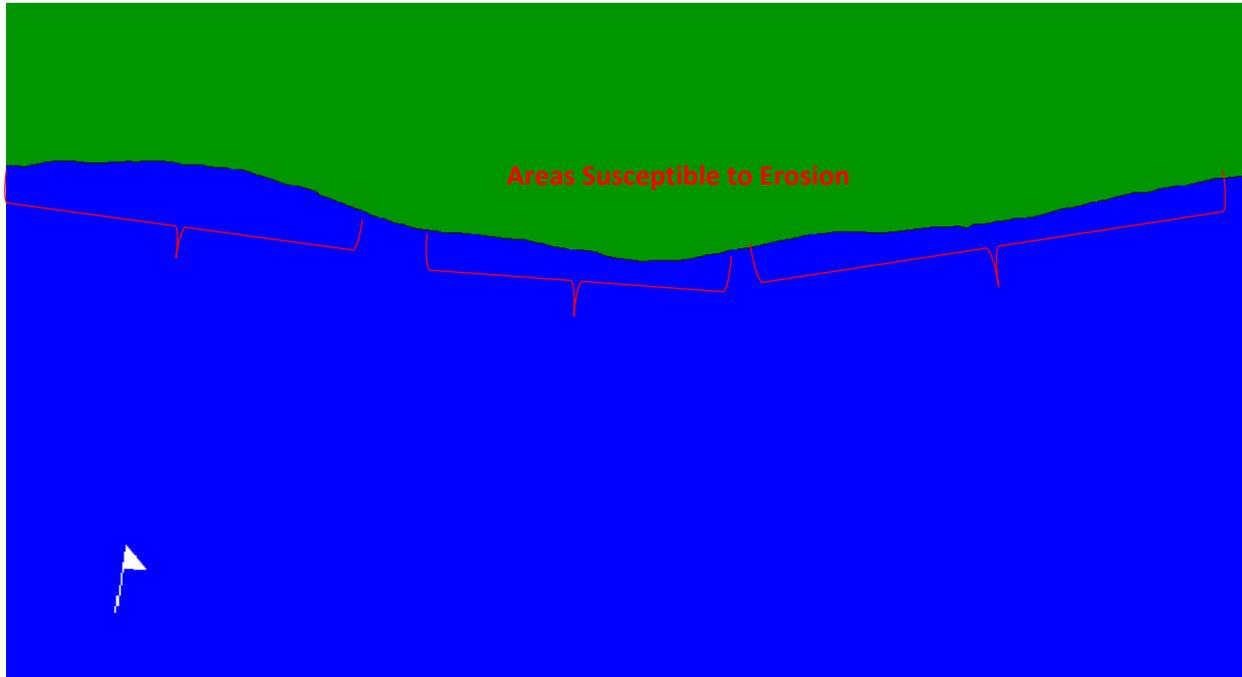
Figure 4.21- Beach planform after 6 years of simulation for the pre-project Palisadoes Caribbean Sea side shoreline
