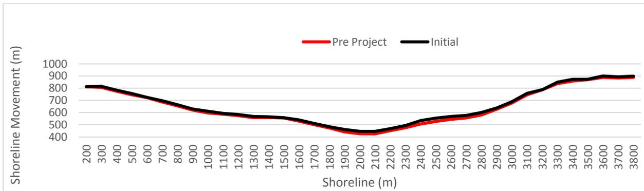
Figure 4.22 Comparative analysis of initial and pre-project shorelines for the Caribbean Sea side of the Palisadoes project
