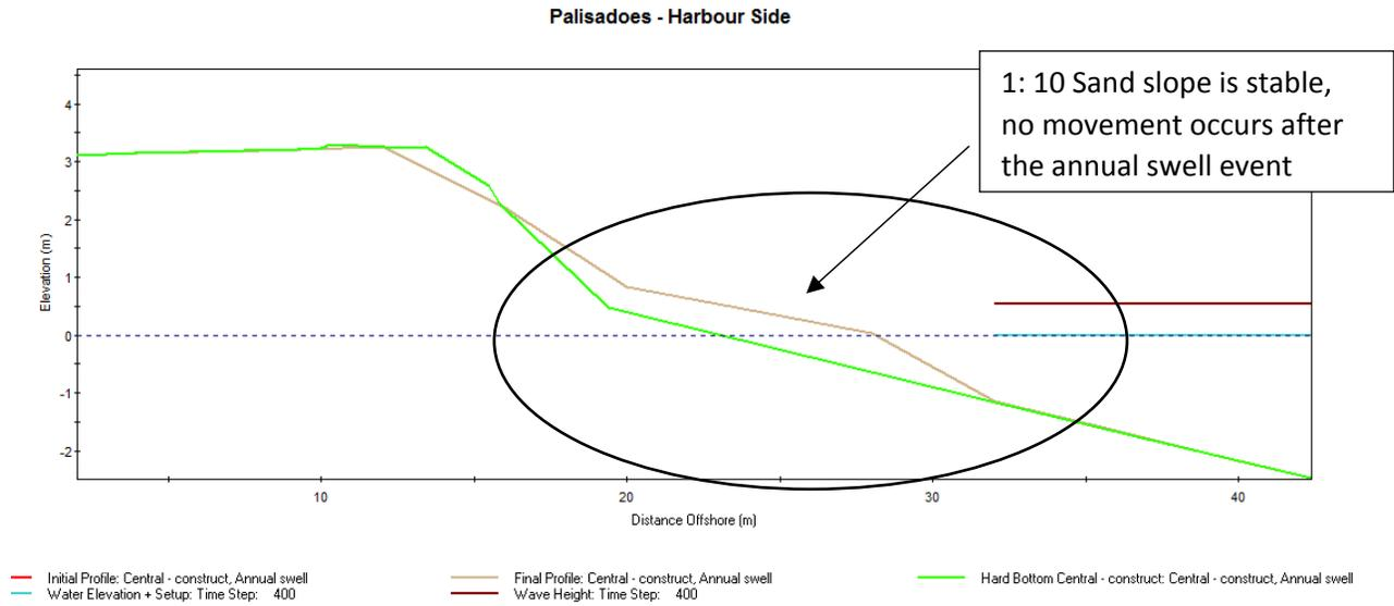
**Figure 4.13 SBEACH results showing the sand placement for mangrove nourishment at the central section of the harbour. The sand is placed at a 1: 10 slope and it doesn't move after the annual swell event, the 1:10 slope is stable**
