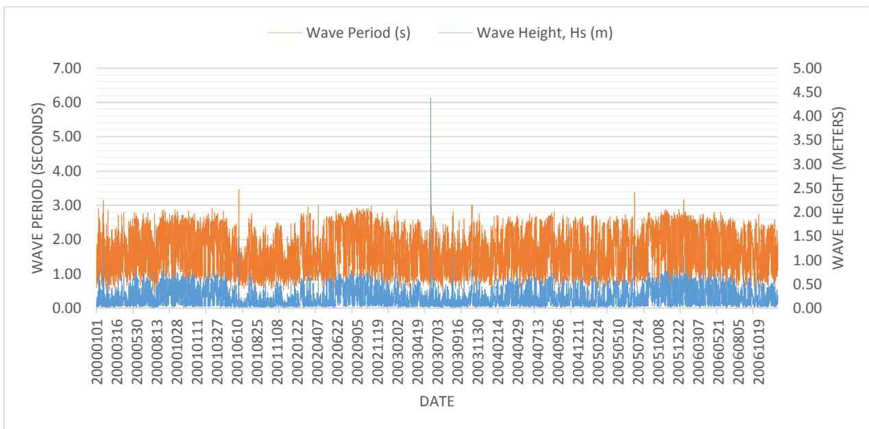
**Figure 4.18 NOAA grib wave data for 2000 - 2006 that was used in sediment transport modeling for the Harbour Side**
