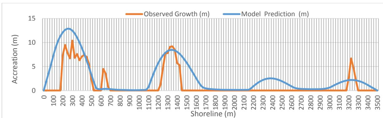
Figure 4.20 Calibration plots for the observed accretion patterns along the Harbour Side Shoreline in comparison to the models (Genesis) predication.
