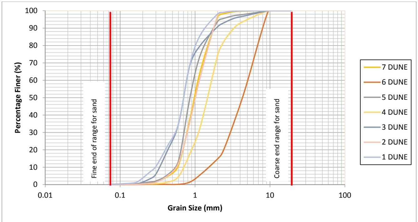
**Figure 2.20 Graph showing the grain size results for the sand taken from the burrow area proposed for the Palisadoes sand dune**
