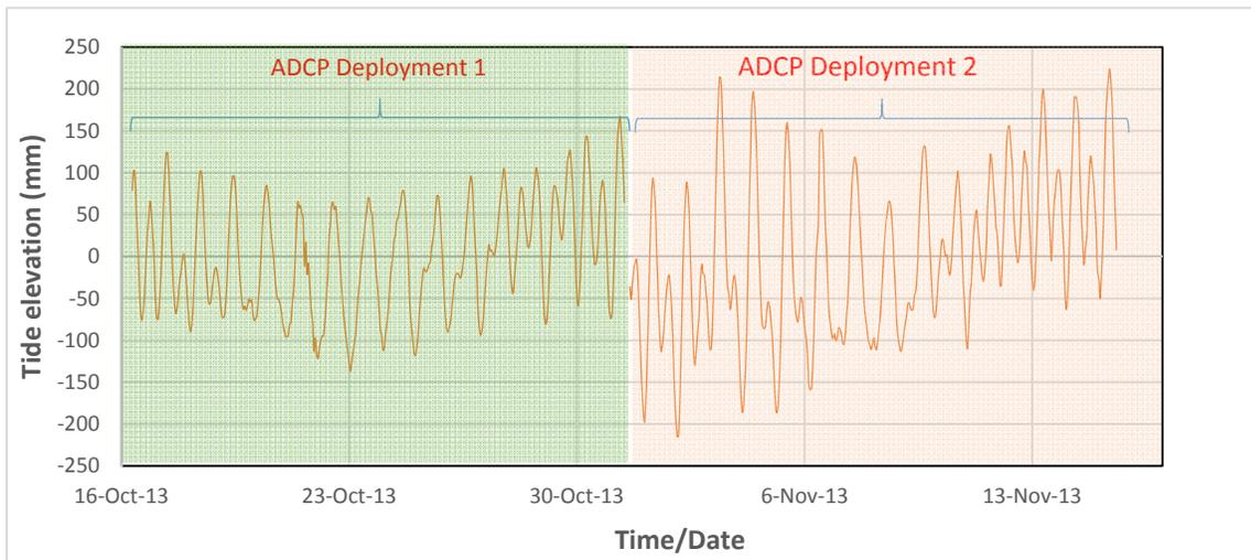
**Figure 2.4 Tidal signal recorded during the ADCP deployment for the period 17<sup>th</sup> of October to 15<sup>th</sup> of November, 2013 for Palisadoes**
