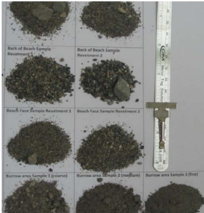
**Plate 2-1** Photograph of sand samples collected from the sand reserve (borrow area) and the shoreline
