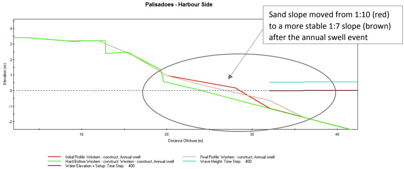
**Figure 4.12 SBEACH results showing the sand placement for mangrove nourishment at the western section of the harbour. The sand is placed at a 1: 10 slope and moves to a 1:7 slope after the annual swell event. The 1: 7 slope is the stable slope for sand in this area.**
