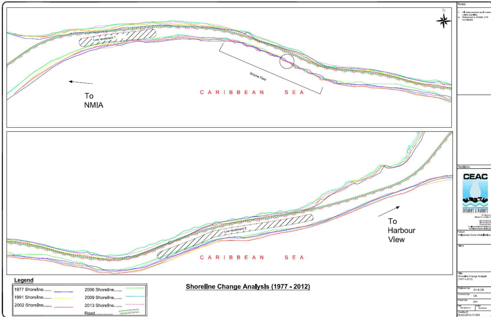
Figure 4.1 Shoreline plots between 1977 and 2013 about the 1968 section for the western section of the Palisadoes closest to the NMIA roundabout (top) and eastern section of the Palisadoes closest to the Harbour View roundabout (bottom)
