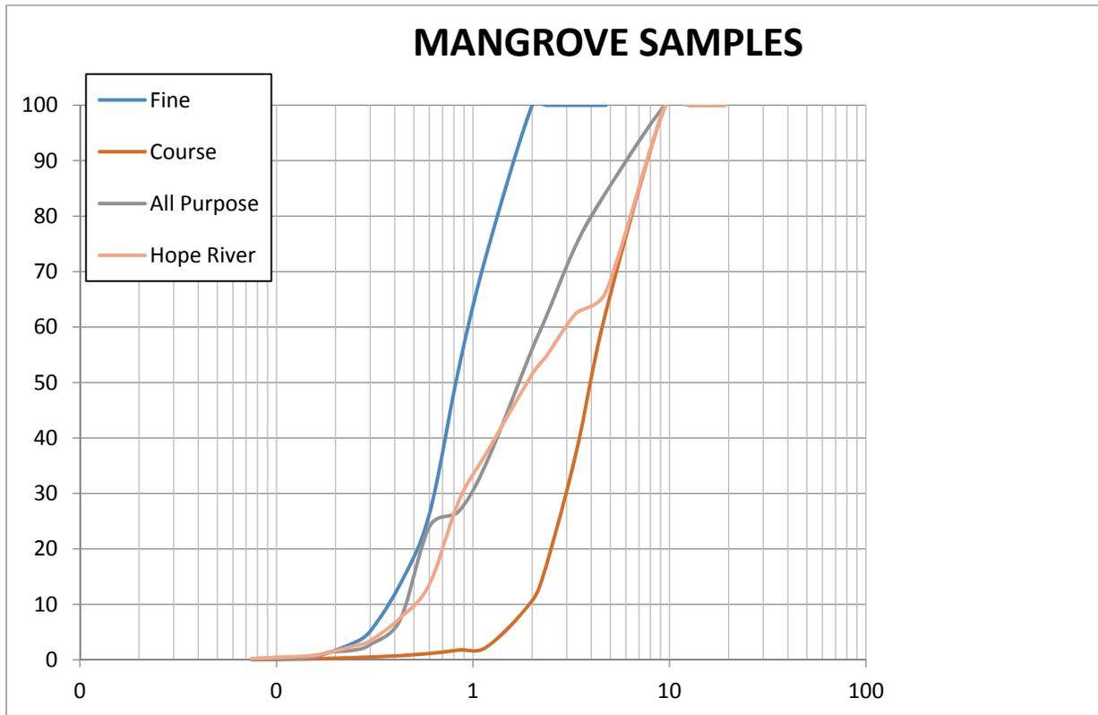
**Figure 2.33 Graph showing the grain size for the sand from the mangrove forest and from the Hope River**
