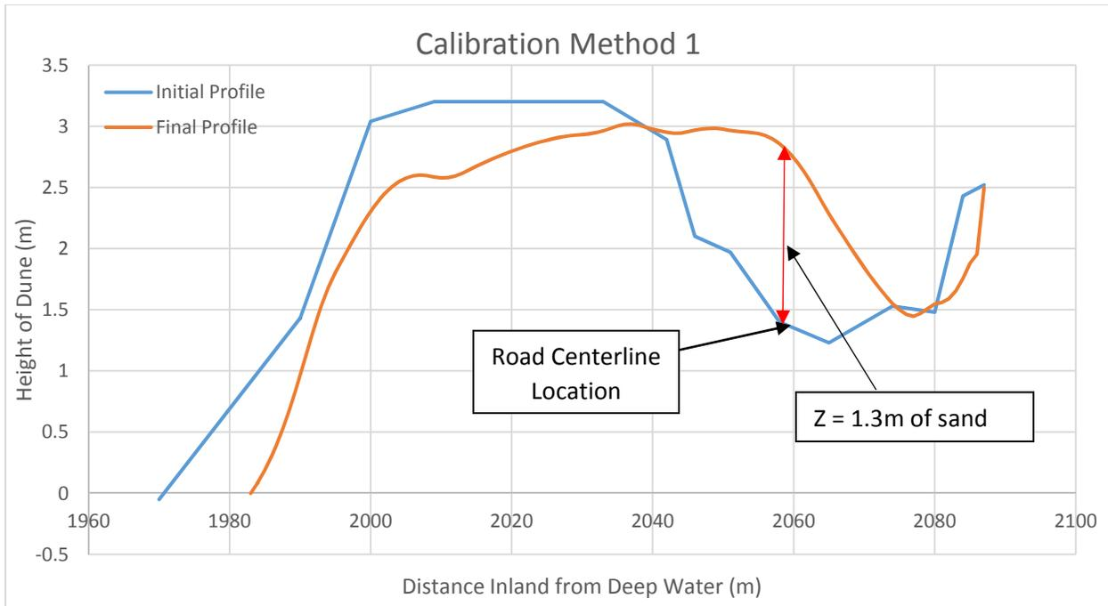
**Figure 4.5 Calibration results comparing observed sand deposition versus model predictions**
