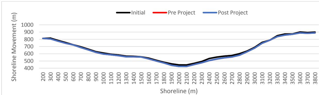
Figure 4.23 Comparative analysis of initial and post-project shoreline for the Caribbean Sea side of the Palisadoes project
