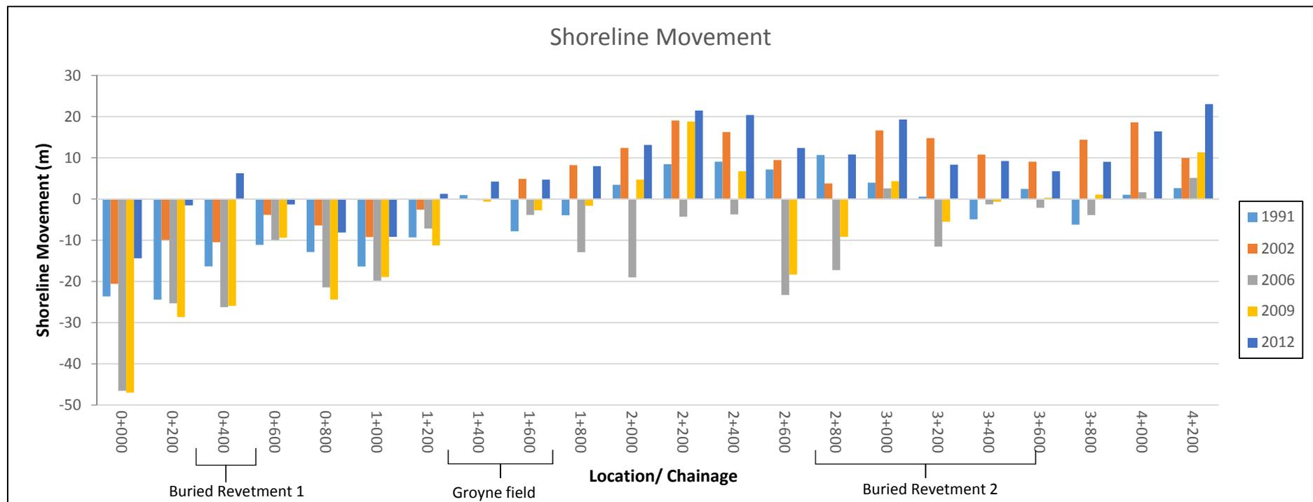
Figure 4.2 Graph showing the displacements of the shoreline for different years about the 1977 shoreline for Palisadoes (1991 to 2012)
