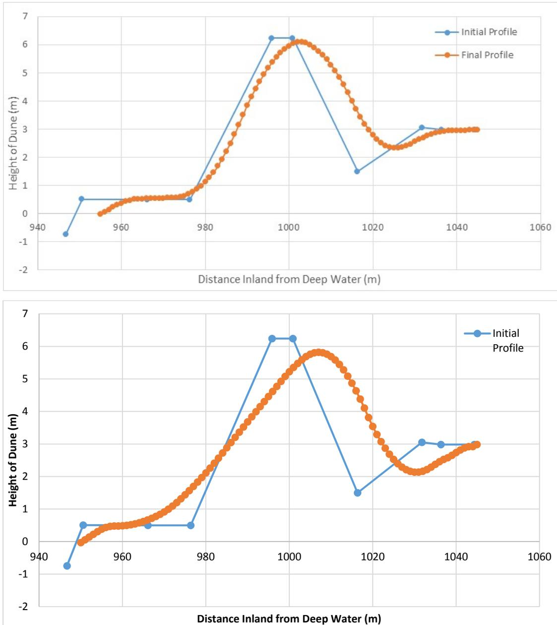
**Figure 4.7 Simulation results comparing pre and post sand dune erosion predictions during 50 (top) and 100 (below) year event**
