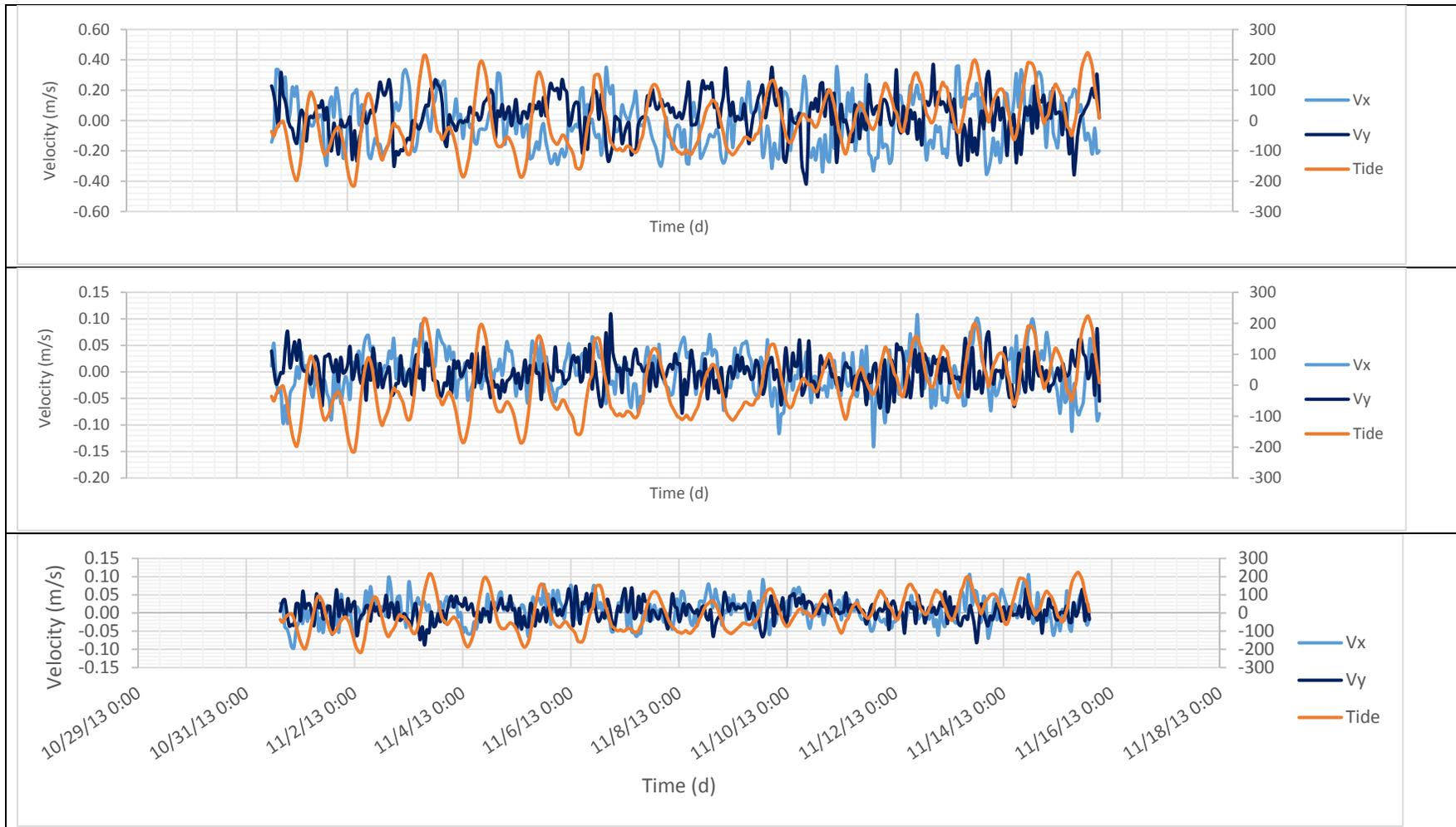
**Table 2-2 Current velocities and tide recordings during the second ADCP deployment of Plumb Point for the surface, mid depth and sea floor respectively**
