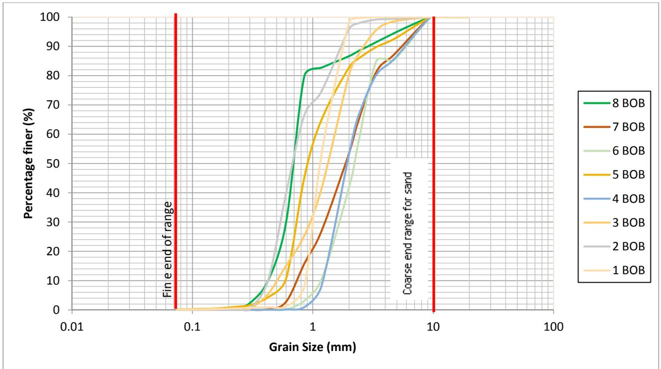
Figure 2.18 Graph showing the grain size results for the sand taken from the Palisadoes along its back of beach (BOB)
