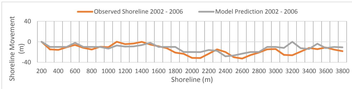
Figure 4.19 Calibration plots for the observed accretion patterns along the Harbour Side Shoreline in comparison to the models (Genesis) predication.
