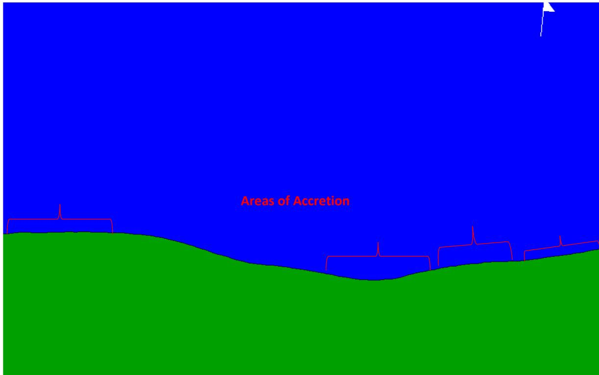
**Figure 4.24 Beach planform after 6 years of simulation for the existing bathymetry and conditions showing pre-project (north arrow shown) along the Palisadoes Harbour Side shoreline**
