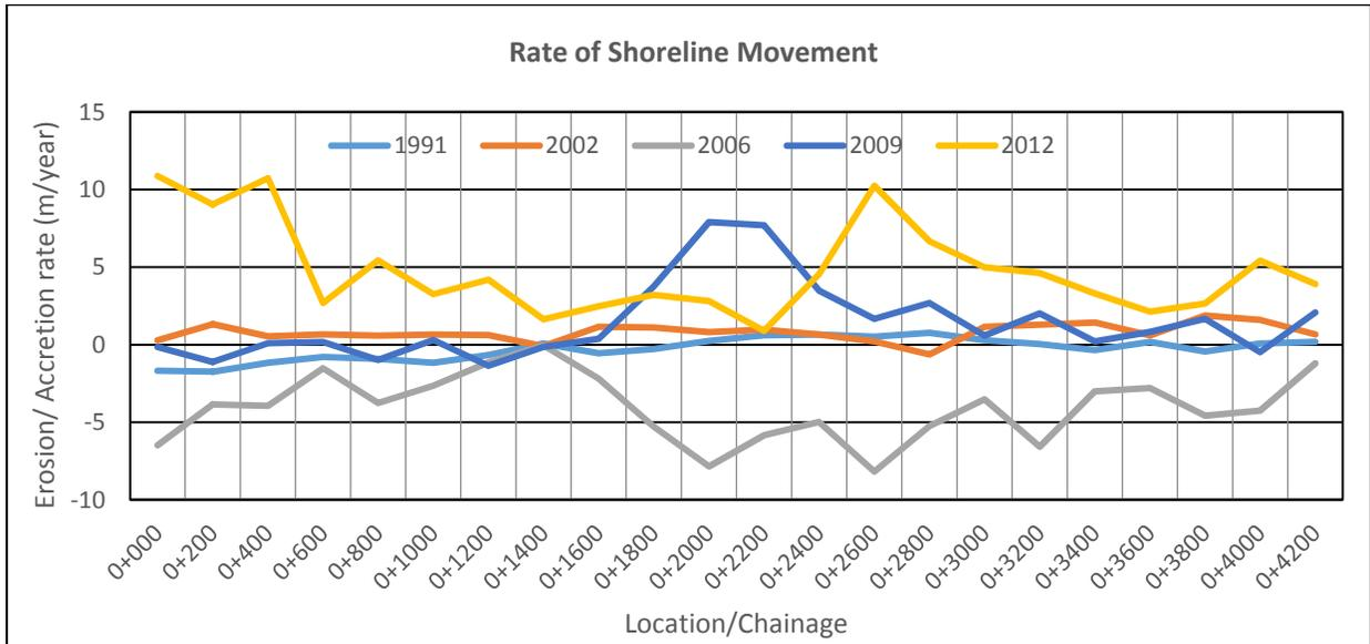
Figure 4.3 Graph showing the rates of erosion/ accretion for the shoreline about the 1968 shoreline for different time intervals between 1991 and 2013. Erosion occurred between 2002 and 2006 because of the passage of hurricane Ivan.
