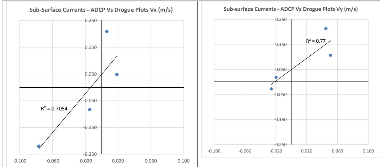
**Table 2-7 Statistical comparison of the currents measured by the drogues and DCP deployed in the Caribbean Sea for the Palisadoes project**
