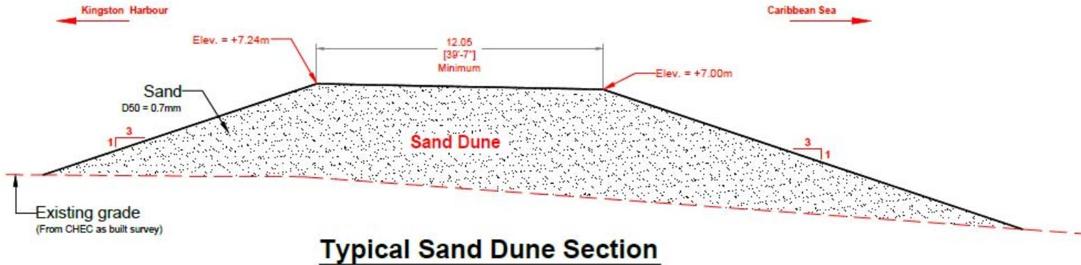
Figure 4.11 Typical section of the sand dune to close the 104 m gap between the high revetment and the NWC WWTP. This is an optional structure to be decided upon by NWA
