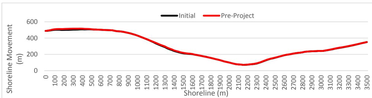
**Figure 4.25 Comparative analysis of initial and pre-project shorelines for the Palisadoes Harbour Side shoreline**
