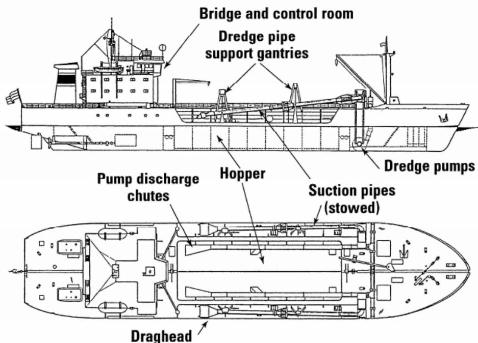
**Figure 6.1 Schematic of Trailing Suction Hopper Dredger**
