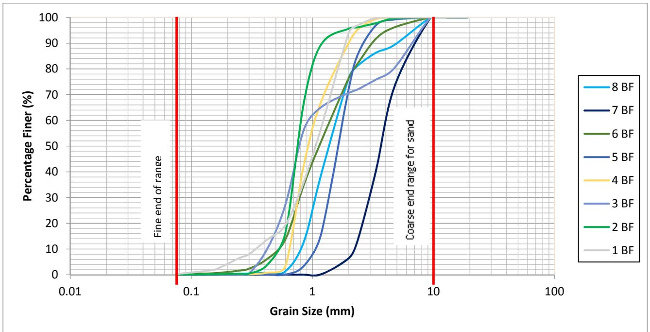
Figure 2.19 Graph showing the grain size plots for the sand taken from the Palisadoes along its beach face (BF)
