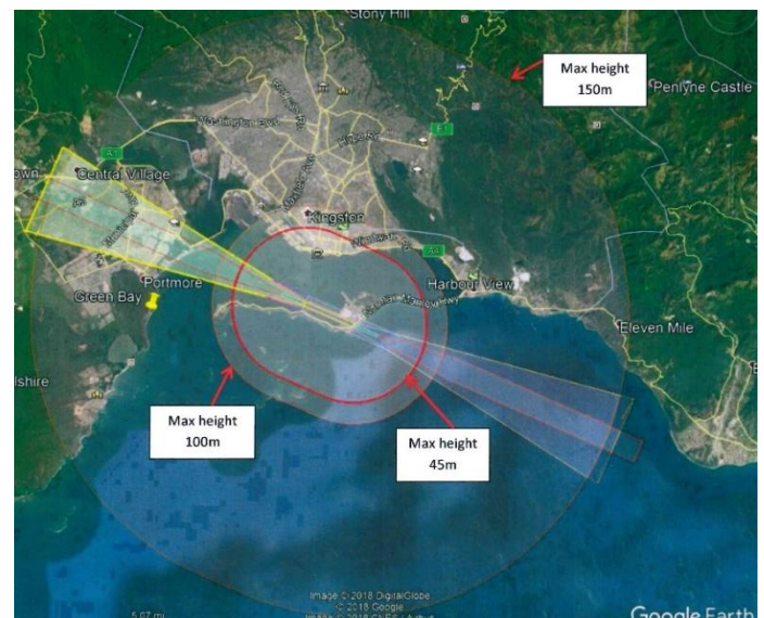
Figure 2.5: Airport Restricted Zones to establish Locality 5
